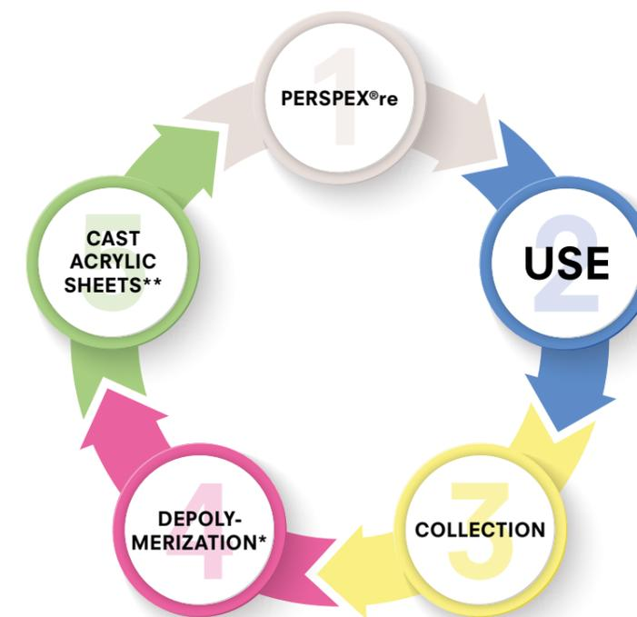
\* **Depolymerization** (Cracking and Distillation – production of rMMA, external waste management)
